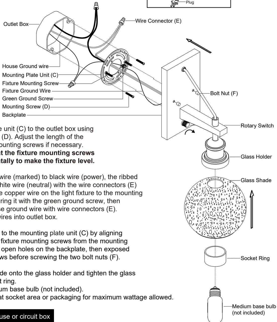
4. Attach mounting plate unit (C) to the outlet box using two mounting screws (D). Adjust the length of the preinstalled fixture mounting screws if necessary.
